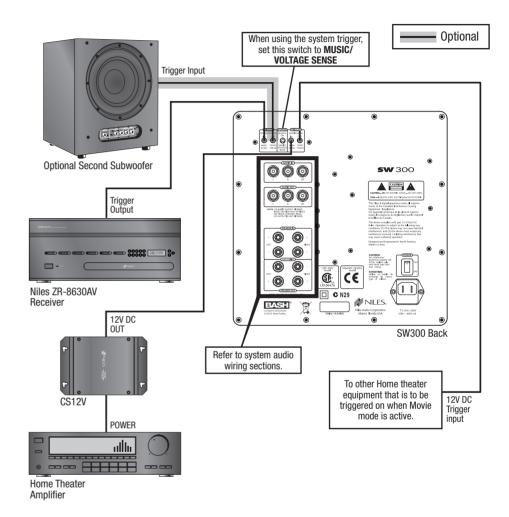
**Figure 6.** Trigger connections
